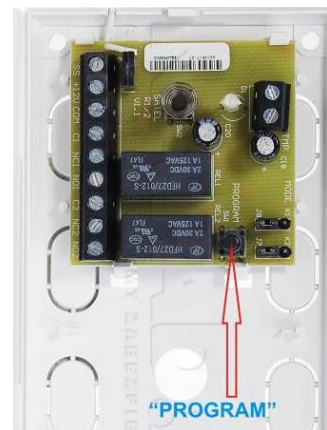
Fig. 14 - Remote control key fobs Satel T-2 Fig. 15 - Radio receiver controller Satel RE-2K
